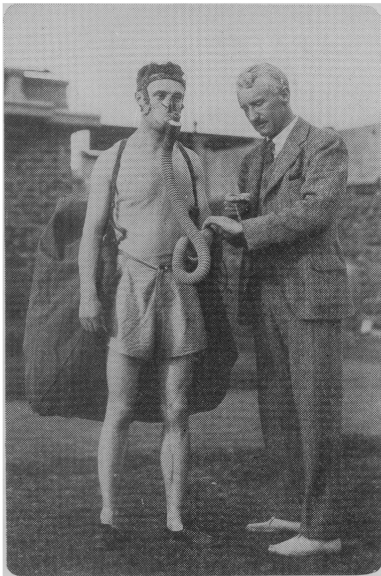
PROF. HILL TAKES THE PULSE of an athlete after running. As he runs he breathes into the bag on his back, and by analyzing the air, to determine dioxide in it, the scientist can measure the rate at which the runner used up his energy.
