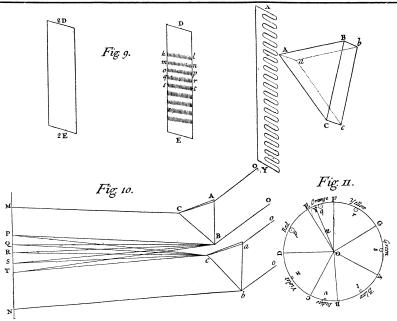
Newton explains his arrangement for obtaining white light from two spectra: "If the most refrangible rays (blue) coming from the superior Prism take up all the space from M to P, the rays of the same sort which come from the inferior Prism ought to begin at P, and take up all the rest of the space from thence towards N"
