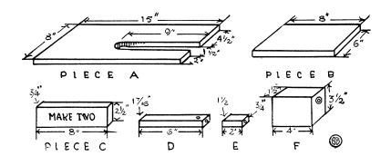
into the end 2 inches deep, and a 5%-inch hole through it the thin way, an inch from the end, and intersecting the 5/16-inch hole. In the large board, piece A, cut a slot  $1\frac{1}{2}$  inches wide and 9 inches long, 2 inches from one edge. All these pieces are illustrated. They may be made of most any kind of wood.
