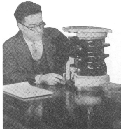
K. B. McEachron and a cut-away lightning arrester containing thyrite, the dual-role substance which he made.
