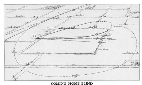
After being guided to the field by the radio range beacon A, the pilot circles the field  $a_{\it n}d$  then glides down the path marked out in space by the runway beacon B and vertically by the landing beam C.
