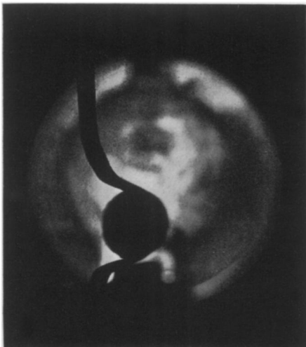
"STOPPING" 240 MILES AN HOUR Ignitron arc-controlling tube of Westinghouse Elec. Co. flashes on for a millionth of a second to "stop" the motion of a rubber ball fired from an experimental gun at velocity of 240 miles an hour. The rubber bullet has struck a rubber sheet on whose surface is a wire. The breaking of the wire by the ball flashes on the new tube and makes possible the photography by its mercury vapor light.
