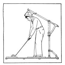
attached to supporting arms that are adjustable according to the golfer's height, holds the head still and in the proper position while the golfer executes his swing. The whole apparatus is supported by a platform on which the golfer stands. With head and feet fixedly in place, the inventor claims that the body is forced to execute the proper pivotal motion, and that practice with this device will obviate the services of a more expensive human instructor.
