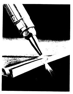
plate at right angles. The torch must be moved very uniformly, for otherwise ridges will be formed. Too much heat and too little heat produce other defects.
