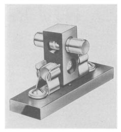
serves also as a handle by which the whole thing can be pulled out, when the operating fuse has blown. The device is then turned over and the spare fuse brought into circuit. The burnt fuse comes out on top where it can be replaced by a fresh one.
