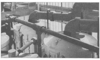
**CLUE No. 1**...The basic raw materials used are—salt, sulphur, sea water, molasses, lead and petroleum gas. This picture shows part of the equipment for evaporating salt brines to produce table salt.
