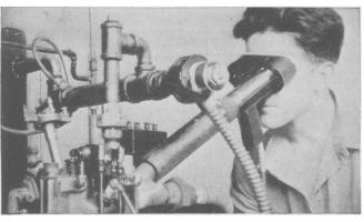
**CLUE No. 4**...This research engineer is using an optical pyrometer to tell, by color, temperature of an exhaust valve in an engine running "wide open." Research is very important in this industry.
