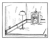
point. The live wires are well buried in recesses under overlying insulating strips and can only be reached by the specially shaped prongs of the movable plug. This invention has just been patented.
