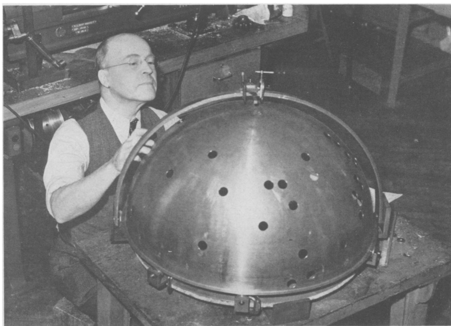
STAR MAKER —Bausch and Lomb has built a new star projector for use by Navy aviators. Men are taught the position and degree of brightness of 145 navigational stars which are projected on the spherical dome. Stars appear realistically in the sky through a period corresponding to a 24-hour cycle, which speeds up instruction. The instrument can be used in the daytime when no stars are visible and can be operated at night when bad weather obscures the stars outside.
