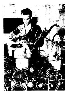
SINGLE-CYLINDER TEST stands are being used at Wright Aeronautical Corporation to speed production of new engines by testing designs in valves, pistons, spark plugs and other parts of the cylinder. Solid plates cover the other cylinder openings in the crankcase. Design features worked out on one cylinder can be applied effectively to a complete engine. This saves time and releases full-sized test cells for use on completed engines ready for installation in planes.
