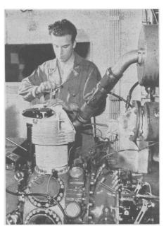
SINGLE-CYLINDER TEST stands are being used at Wright Aeronautical Corporation to speed production of new engines by testing designs in valves, pistons, spark plugs and other parts of the cylinder. Solid plates cover the other cylinder openings in the crankcase. Design features worked out on one cylinder can be applied effectively to a complete engine. This saves time and releases full-sized test cells for use on completed engines ready for installation in planes.
