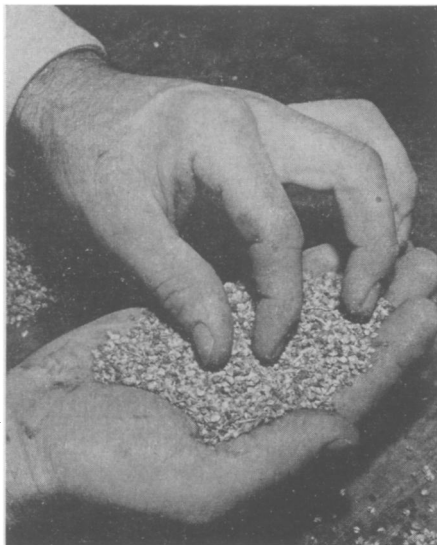
WORMS —That is what the guayule rubber is called when it is in this form after being chopped and crushed and put in settling tanks.
