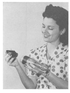
huge quantities, the saving of aluminum is considerable. The plastic used was specially developed for the purpose. It had to be extra hard, and maintain its dimensions accurately in all weathers.
