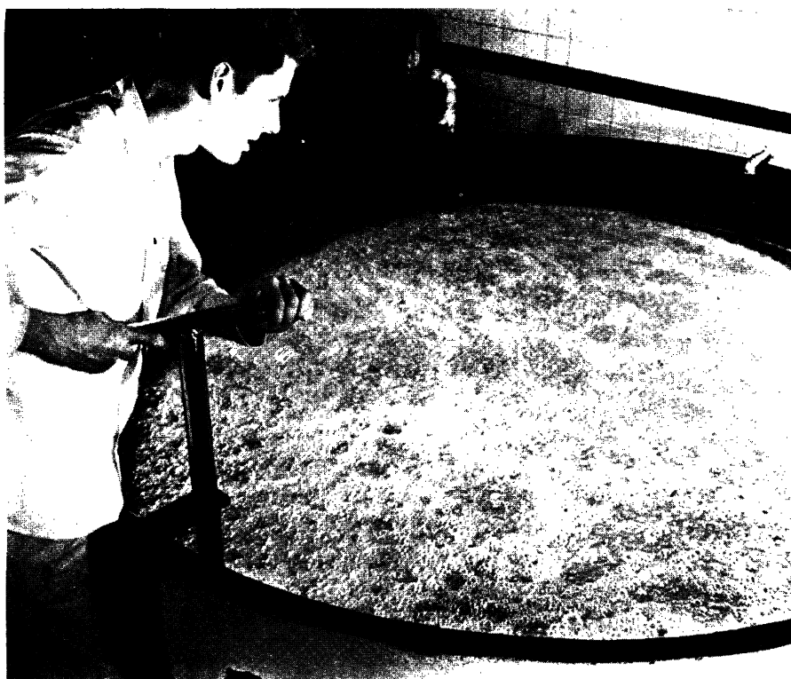
CONVERTED —Scene in a whiskey distillery now making industrial alcohol. The operator is opening a valve to add yeast to the mash in a fermenting tank. This is an official photograph of the Office of War Information.
