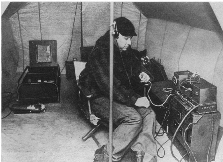
BRIDGING GAP —This radio telephone unit spanned the Hudson River after a vessel severed underwater cables.
