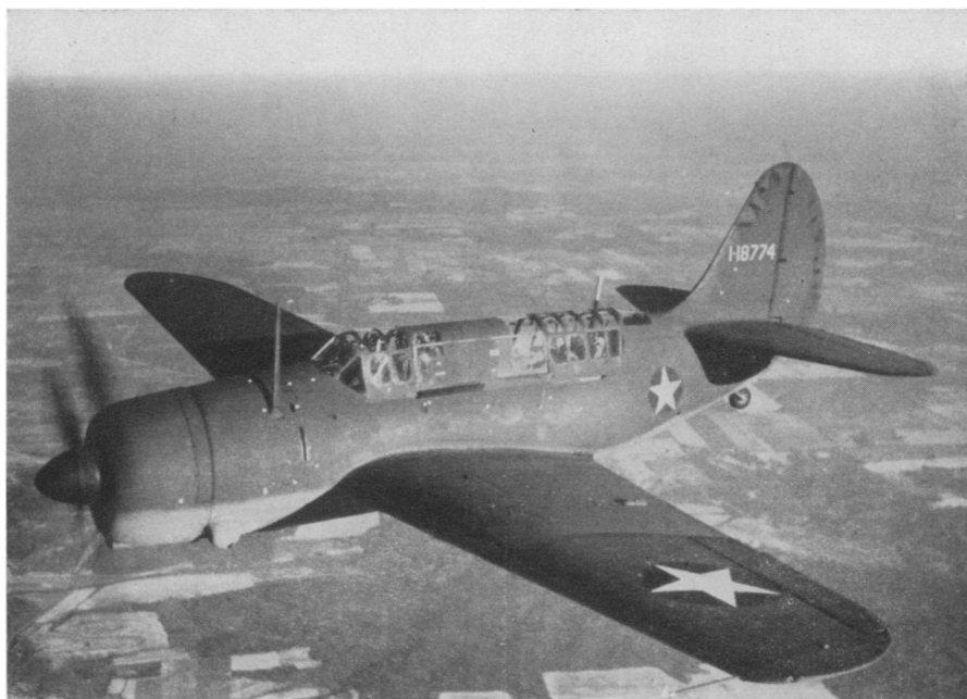
NEW HELLDIVER —This new Curtiss A-25 is a two-place, mid-wing monoplane powered with a 1700-horsepower Wright Cyclone Engine and equipped with a three-bladed Curtiss electric propeller and retractable landing gear. Just what it can do is kept secret, but the manufacturer claims that it has greater speed, range and striking power than any other dive-bomber now in action. Quantity production on a continuously moving assembly line is now under way.
