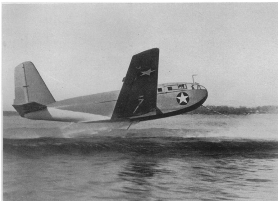
AMPHIBIOUS —Transport glider, America's newest invasion weapon, was made for the U. S. Navy of molded plywood and other non-strategic materials by Allied Aviation Corporation.
