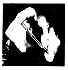
MERCURY LAMP — Scarcely bigger than a wooden match, this small mercury lamp developed by the General Electric Company is good for one million photographic exposures.
