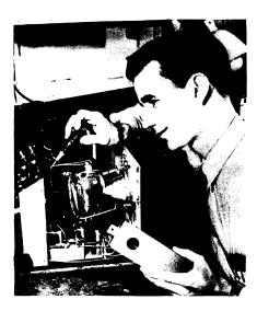
FLASH PHOTOGRAPHY—The inside of a portable millionth-of-a-second flash light for photography is being shown by S. L. Bellinger, a General Electric engineer. The phototube accessory equipment which may be used in fast operation of the light is held in his left hand.
