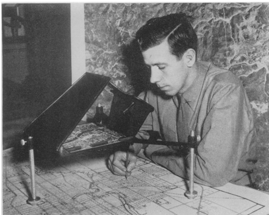
BETTER MAPS —The soldier, using photographs made from airplanes, constructs and corrects maps by use of the Abrams Vertical Sketchmaster, which adjusts the pictures to the proper scale.
