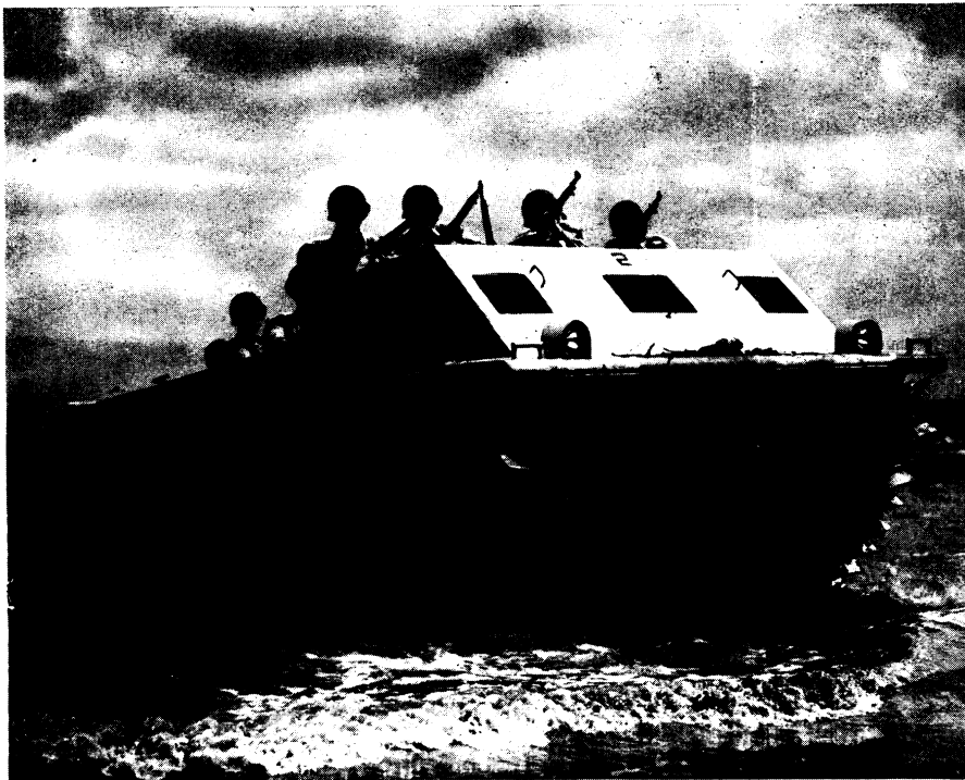
"ALLIGATOR"—This amphibious tractor developed for use by the U. S. Marine Corps in landing operations combines the features of a tank and armored landing boat. The dual vehicle protects men and vital equipment in landing on a hostile shore as well as in crossing swampy terrain.
