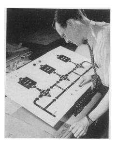
PIPELINE NURSE — A few pushbuttons will control the flow of millions of gallons of vital oil products through the 20-inch pipeline now being built between Houston, Texas, and the Eastern Seaboard. For each of the line's 29 pumping stations Westinghouse Electric & Manufacturing Co. is building an electrical "nurse" consisting of a control desk with a diagram of which this is a model.
