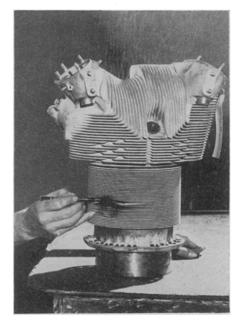
BULLET-RIDDLED — Experts are studying this Wright Cyclone engine cylinder, back from "somewhere in the Pacific" (See SNL, May 23, 1942). The ragged hole is where a 50-caliber enemy bullet completely pierced the cylinder barrel. In spite of the puncture, the tough engine
