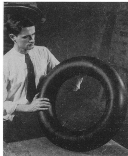
PLASTIC TIRE — An inner tube made from Marvinol being inspected by Clayton F. Ruebensaal, of the Glenn L. Martin Plastics Research Laboratory, who, with Earl H. Sorg, developed this new elasto-plastic.
