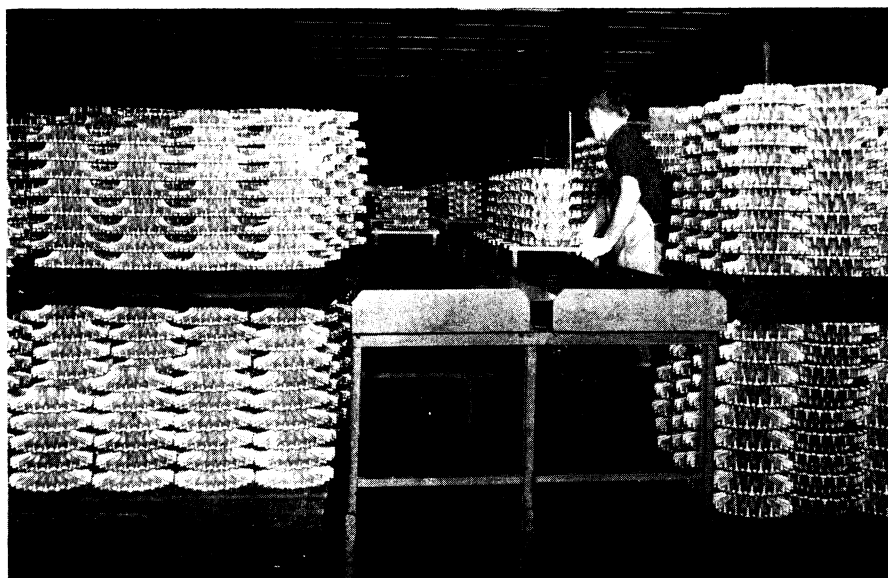
FOR STRATOSPHERE —These are supercharger impellers, "fan" blades for the bombers that will fly in the upper air over enemy territory. They are being built in General Electric's Fort Wayne, Ind., plant.
