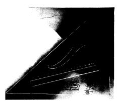
VERSATILE — This draftsman's tool, made of "Lumarith," includes among other features markings for a ten-inch rule; a straight edge; angles of 15, 30, 45, 60, 75 and 90 degrees; a French curve; graduation markings; and holes for use in drawing parallel lines.
