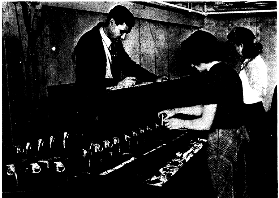
X-RAY CHECKER —A hand grenade will explode prematurely if the powder charge is less than the required amount. To prevent this, the General Electric Company devised this machine to check the powder charge in each fuse. When a bad fuse is found by an electric eye, a bell rings, a red lamp is lighted, a dab of red paint is placed on top of the bad fuse and a recording is made on a chart. Four thousand tubes pass through the machine in an hour.
