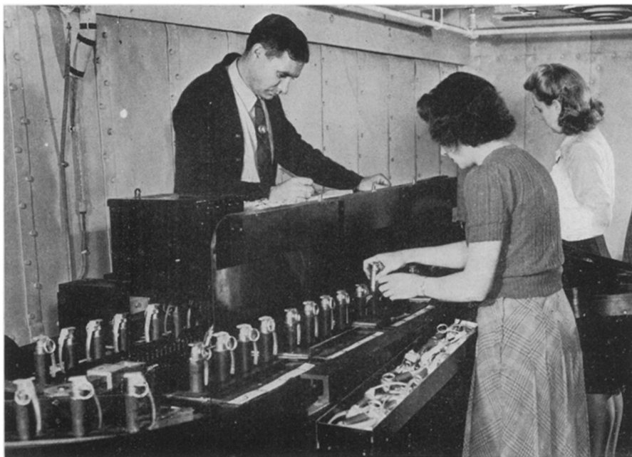
X-RAY CHECKER —A hand grenade will explode prematurely if the powder charge is less than the required amount. To prevent this, the General Electric Company devised this machine to check the powder charge in each fuse. When a bad fuse is found by an electric eye, a bell rings, a red lamp is lighted, a dab of red paint is placed on top of the bad fuse and a recording is made on a chart. Four thousand tubes pass through the machine in an hour.
