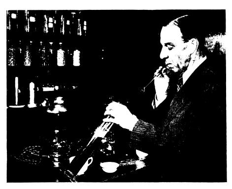
COFFEE BREW—To determine the percentage of extraction in a coffee brew, Prof. Backer first draws 50 cc. of the brewed coffee into a pipette, from a measured amount of the brew. The coffee is emptied into a porcelain dish and placed in an oven where the heat drives away the water. After it is cool, the coffee extract remaining in the dish in solid form after the evaporation is measured with a delicate balance to calculate the percentage of extraction.
