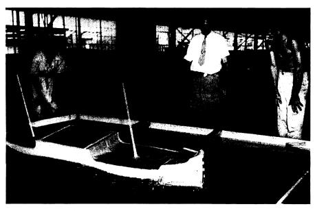
MODEL LAUNCHING—The narrowness of the Tennessee River at Decatur, Ala., makes it necessary for the Ingalls Shipbuilding Corp. there to resort to side launchings. While a ship is still in the blue print stage, a sixfoot model is constructed and tested out in a tank which approximates, proportionately, the river's width. After it has hit the water, the model is closely observed for heel-over and the distance it floats before coming to rest.
