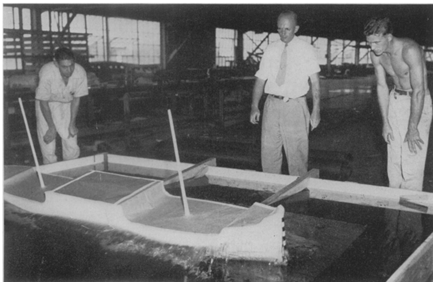
MODEL LAUNCHING —The narrowness of the Tennessee River at Decatur, Ala., makes it necessary for the Ingalls Shipbuilding Corp. there to resort to side launchings. While a ship is still in the blue print stage, a six-foot model is constructed and tested out in a tank which approximates, proportionately, the river's width. After it has hit the water, the model is closely observed for heel-over and the distance it floats before coming to rest.
