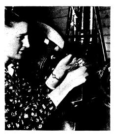
TESTING BOMB FUZE—A fuze for a 20-pound fragmentation bomb is being installed in the path of a man-made gale to determine how the fuze would perform when dropped by an American airman. Wind tunnel tests such as this at the Westinghouse East Springfield plant provide a constant check on the quality of fuzes produced.
