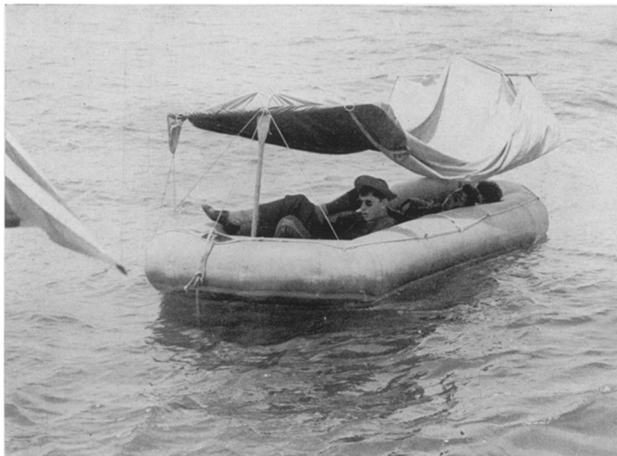
TARPAULIN CANOPY —Results of tests carried out by nine Air Force men showed that those who did not rig up over them some sort of covering to protect them from the blistering rays of the sun felt the effects of dehydration considerably more than the men on the covered raft.
