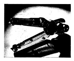
\*DOUBLE-EDGED razor blades are quickly sharpened with a small abrasive block slightly hollowed lengthwise. A shelf and guard in the center prevent sidewise movement while the blade is pushed forward and back. A patent has just been issued.
