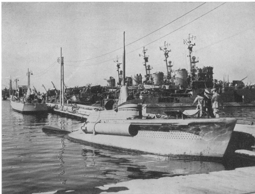
ITALIAN MIDGET —One of the tiny submarines of Italy's fleet is shown in this official U. S. Navy Photograph. Below the torpedo tubes fixed to the sides, the hull bulges out, making it look like a turnip from a bow-on view.
