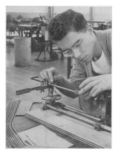
used daily in aircraft factories will make any bend or rotation within a half degree of accuracy. The simplicity of the machine is shown in the picture. The bending arm on the left has a pointer and a plate marked in degrees below.
