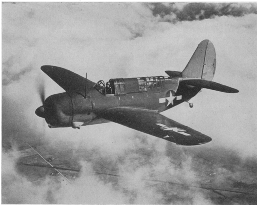
HELLDIVER —This low-mid-wing monoplane, the latest of the Curtiss-Wright Helldiver series, proved its value in the attack against the Japanese stronghold at Rabaul in November. It was designed to carry a greater bomb load faster and farther than any similar aircraft type in the world. The bomb load is housed entirely within the belly of the fuselage, making the lines of the fuselage as aerodynamically clean as possible.
