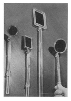
The thumb of the inspector pressed against a knob on a small rod attached to the light plastic handle quickly turns the mirror at varying angles to its handle. The picture shows several types of mirrors and handles.
