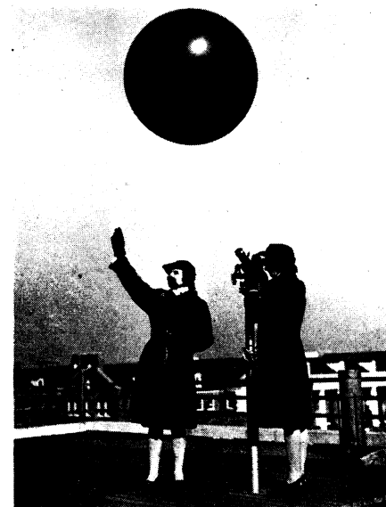
AIR WAVES —The part these two WAVES are playing, in manning the shore jobs so that men can be released for the fighting fronts, is a highly technical one. The aerographer's mate (left) is losing a pilot balloon at the Naval Air Station, Anacostia, D. C., while the officer aerologist (right) prepares to follow the path of the balloon with a theodolite. Their study of atmospheric conditions is essential for maintenance of an air station. Official U. S. Navy photo.
