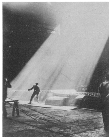
UNDER THE SUN —As a preliminary operation in steel plate production, this workman is turning a slab broadside preparatory to further rolling on a sheared plate mill of the U. S. Steel Corp.
