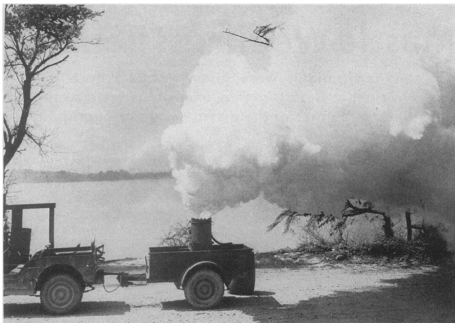
SMOKE-SCREEN —With a portable fog generator the Army can carry large-area smoke screens to beachheads, mountain passes and jungle trails. With favorable conditions, this one generator can blot out an area five or six miles long and 200 yards wide.
