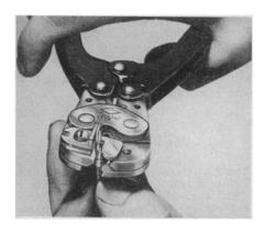
tric wiring without the use of solder or heat. Pressure on the handles crimps the terminal connections to form a strong joint which offers little electrical resistance and resists corrosion.
