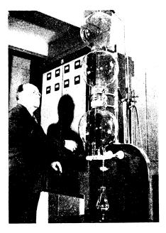
SAVES TIME—Life-saving penicillin is produced much faster when the solutions are dried with this new electronic installation, shown with its inventor, Dr. George H. Brown, research engineer of RCA Laboratories.
