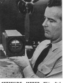
ATTITUDE METER—This little gyro instrument tells the pilot which way is up and at what strange angle his plane is with reference to the surface of the earth. Thus, he can perform all aerobatic maneuvers without seeing the horizon.
