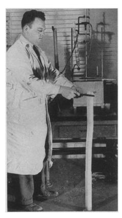
"GROWING" PLASTIC — Foam plastic that "grows" faster than corn promises to have many uses in insulation. Placed in a test tube in General Electric's laboratory, it begins immediately to "grow" at the rate of more than an inch a second.
