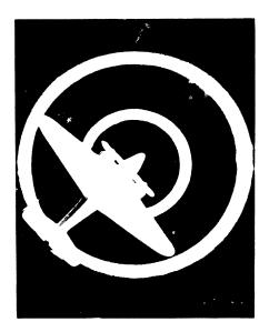
CLEAR VIEW—Here is what a gunner sees when he aims at an enemy plane through a sight equipped with a new Westinghouse gunsight lamp. The sight lines stand out bright and clear, making it possible to fire accurately even while aiming directly into the sun. Without this lamp the gunner could not aim within about 15 degrees of the sun, thus leaving a dreaded blind spot from which the enemy could dive to attack.
