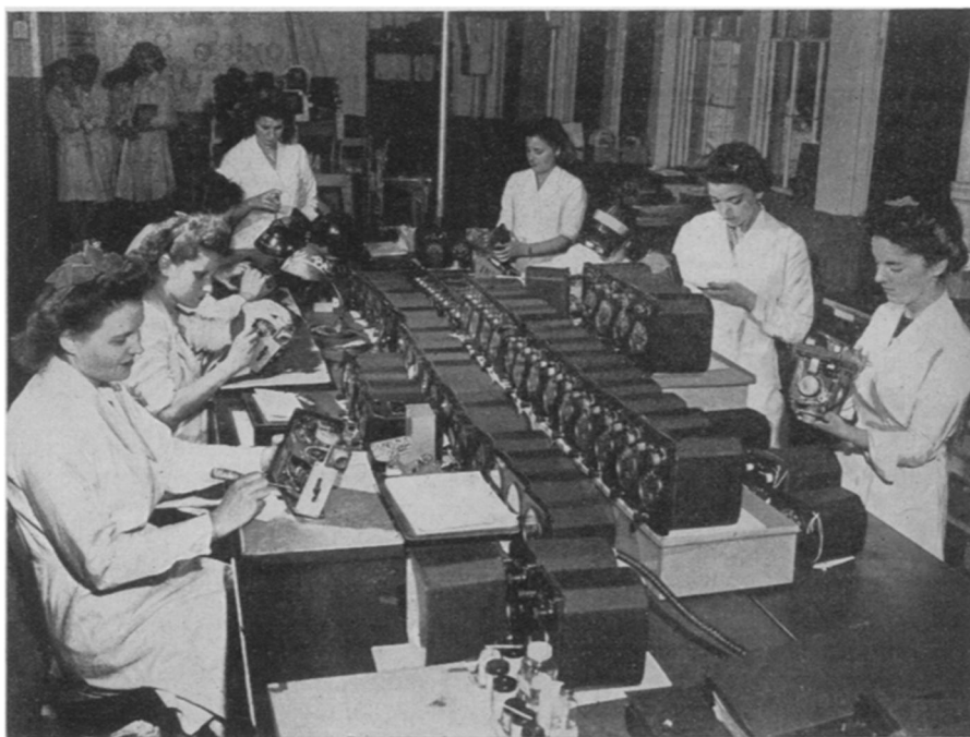
STABILIZERS —The girls in this General Electric laboratory are giving a final inspection to gyroscopes before they are sent to the Army and Navy for use as balancers while planes are in flight.
